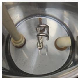
After water treatment via IPS KalyxX 100.
